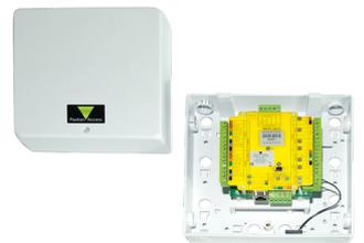
**P31128P.PLUS****Net2 Plus Controller, nur Platine, RS485-TCP/IP**
